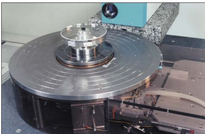
Angle comparator, measuring step approx. 0.001"
